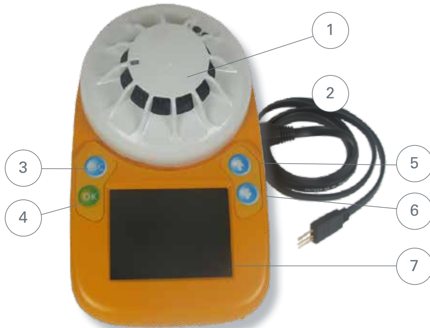
Top View 1 - Detector on Tool Base Twist detector clockwise to engage and lock in position 2 - Ancillary Lead Used for programming MX devices 3 - Escape Button 4 - OK Button 5 - Up Arrow Button 6 - Down Arrow Button 7 - LCD Touch Screen
